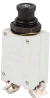
Single pole, miniaturised, aircraft style thermal circuit breaker with tease-free, trip-free, snap action mechanism and push/pull on/off manual actuation. An indicator band on the push button clearly shows the tripped/off position. Threadneck panel mounted. Temperature compensated from -55° to +125 °C, with optional auxiliary contacts, and fully approved for use on a wide range of aircraft and equipment.
