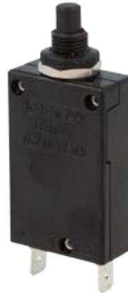
Single pole thermal circuit breaker with press-to-reset, tease-free, trip-free, snap action mechanism. Equipped with threadneck panel mounting. The circuit can be interrupted by push-push action.
