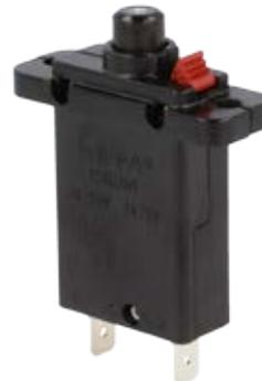
Single pole thermal circuit breaker with press-to-reset, tease-free, trip-free, snap action mechanism. This switch has a manual release option as well. The circuit can be interrupted by push-push action.
