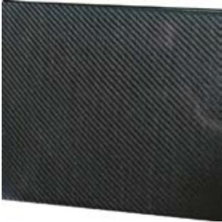
Fiberglass plate, with 1 layer carbon. 1mm thick.
